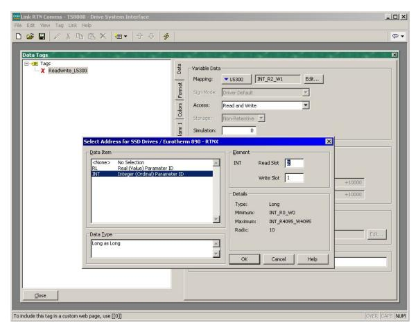
The Read Write tag uses the L5300 (Node 500) device mapping, since that is the destination device for the data. It specifies both Write Slot 1 and Read Slot 2, since those are the data slots that were programmed at the L5300. Keep in mind that in this scenario, reads are ALWAYS implied to be from the Host node.
