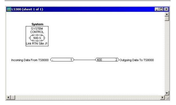
The L5300 is programmed with the Incoming and Outgoing Slots to send and receive data to and from the TS8000.
