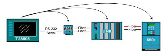
**How The TS8000 Reads Data From Link** – Data going to the TS8000 may only be written to the HOST device on the Link network. The TS8000 data tag uses the source device mapping of the Host to specify exactly where the data is coming from.
