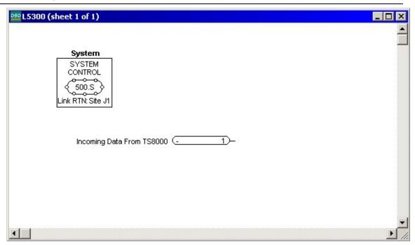
The L5300 is programmed with the Incoming Slot to receive the data from the TS8000. This data is passed from the TS8000 via the Host TechBox (Node 400) to the L5300 (Node 500). This data is now available to use as needed in the Link application.
