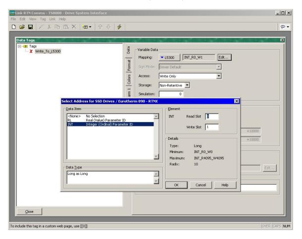
The Write Only tag uses the L5300 (Node 500) device mapping, since that is the destination device for the data. It specifies Write Slot 1, since that will be the incoming data slot that we will program at the L5300.
