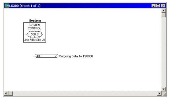
The L5300 is programmed with the Outgoing Slot to send data to the TS8000. This data is sent to the Host TechBox (Node 400) and then read serially by the TS8000. You do not have to explicitly define an Input Slot in the Host TechBox for this data.
