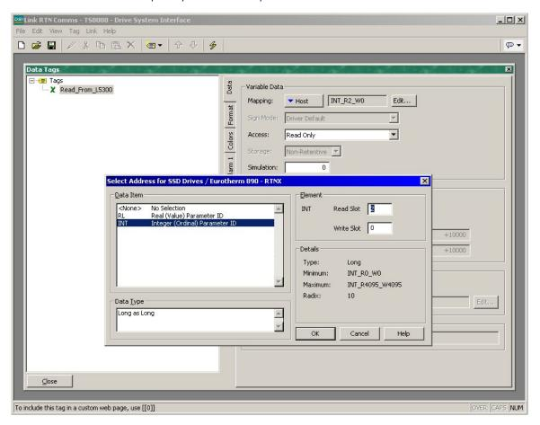
The Read Only tag uses the Host (Node 400) device mapping, since that is the source device for the data. It specifies Read Slot 2, since that is the outgoing data slot that was programmed at the L5300.
