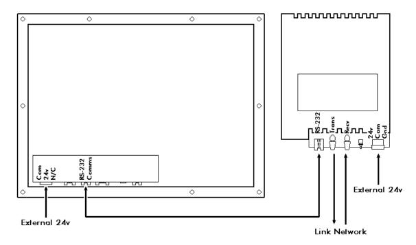
Connect external 24v DC power to both the TS8000 and the 8000/LK/00.
