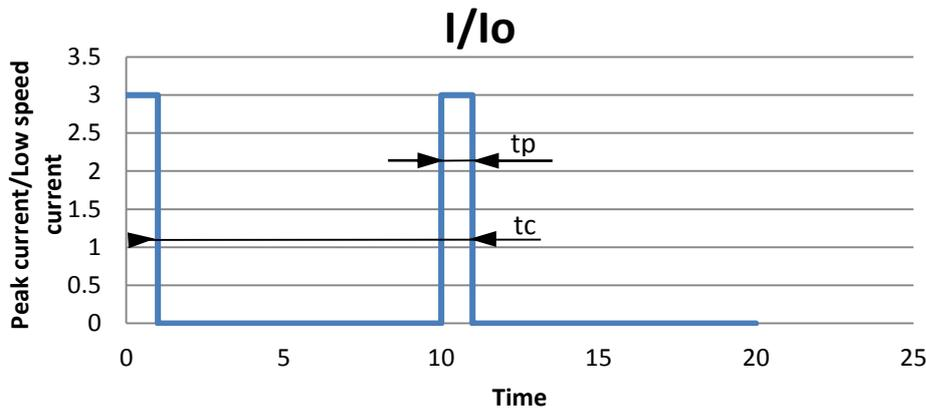
It is possible to use the SKW motors with a current higher than the permanent current. But, to avoid any overheating, the following rules must be respected.
