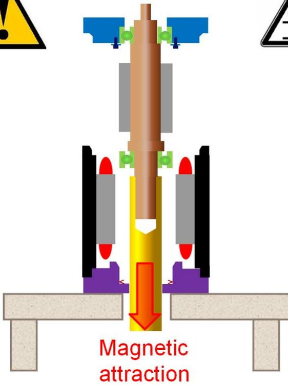
Danger : do not put your hand inside the motor during way-down.
