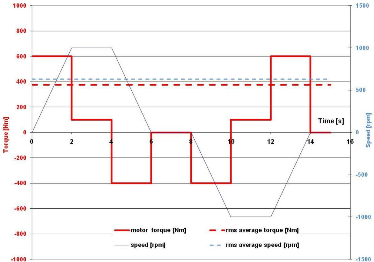
The maximal torque  $M_i$  delivered by the motor at each segment  $i$  of movement is obtained by the algebraic sum of the acceleration-deceleration torque and the resistant torque. Therefore,  $M_{max}$  corresponds to the maximal value of  $M_i$ .
