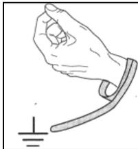
Warning: KTY sensor is sensitive to electrostatic discharge. So, always wear an antistatic wrist strap during KTY handling.
