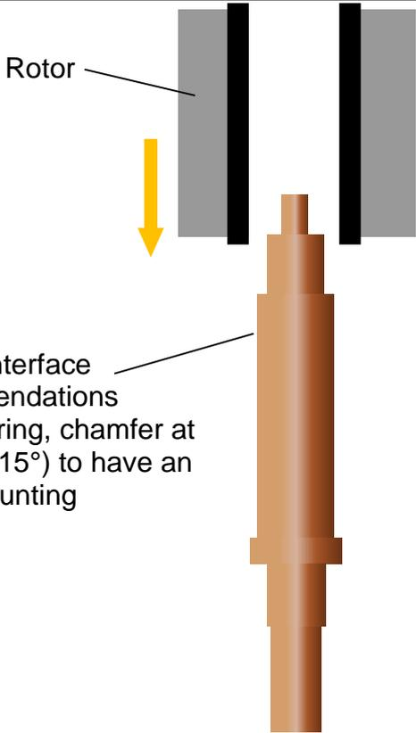
Push down the rotor on the shaft
