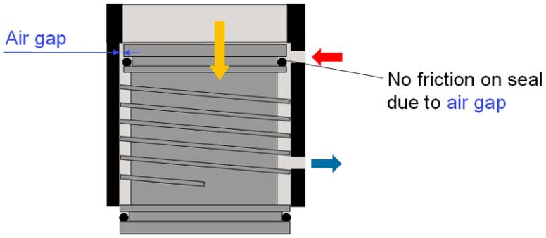
Push down the cooling jacket on the water jacket.
