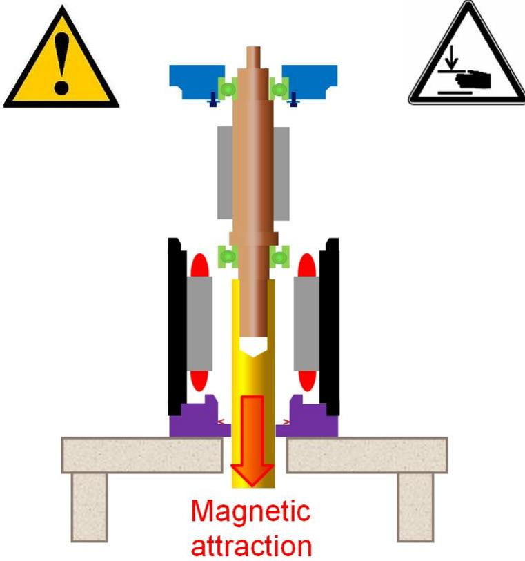
**Danger** : do not put your hand inside the motor during way-down.
