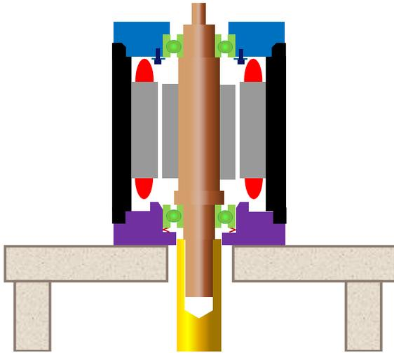
Screw the rear flange on the stator to close motor.
