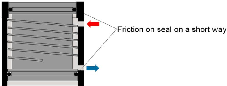
Cooling jacket instructions have been designed to minimize the O-Ring seal friction.
