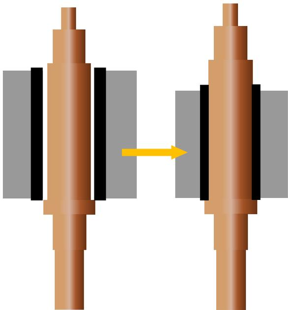
After fitting, let rotor+shaft go back to ambient temperature
