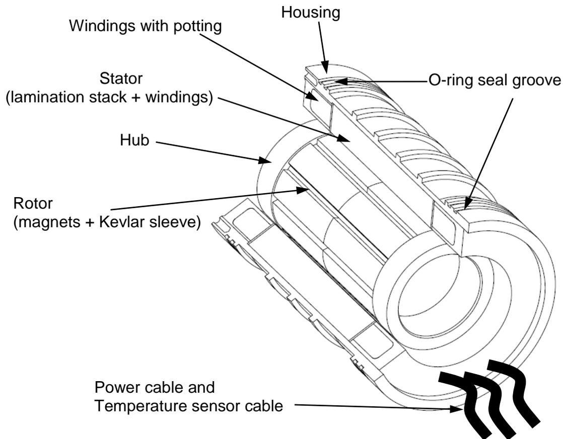
These components are typically assembled according to Figure 1 to make a complete motor spindle unit. The stator is water cooled to allow a higher torque density and a lower stator temperature rise. The motor is designed to have a large shaft diameter to increase the mechanical rigidity.
