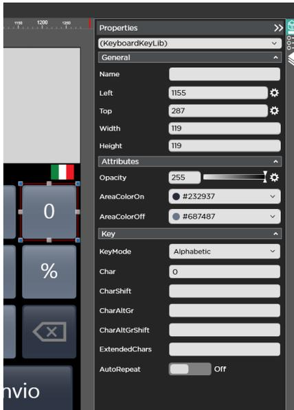
For each softkey the user can define both the graphic layout (key pressed colour, key released colour, font) and the scancode code with all the combinations.
