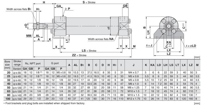
\* Foot brackets and plug bolts are installed when shipped from factory.
